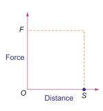
The area under the force versus distance graph is numerically equal to the work done by the agent.
